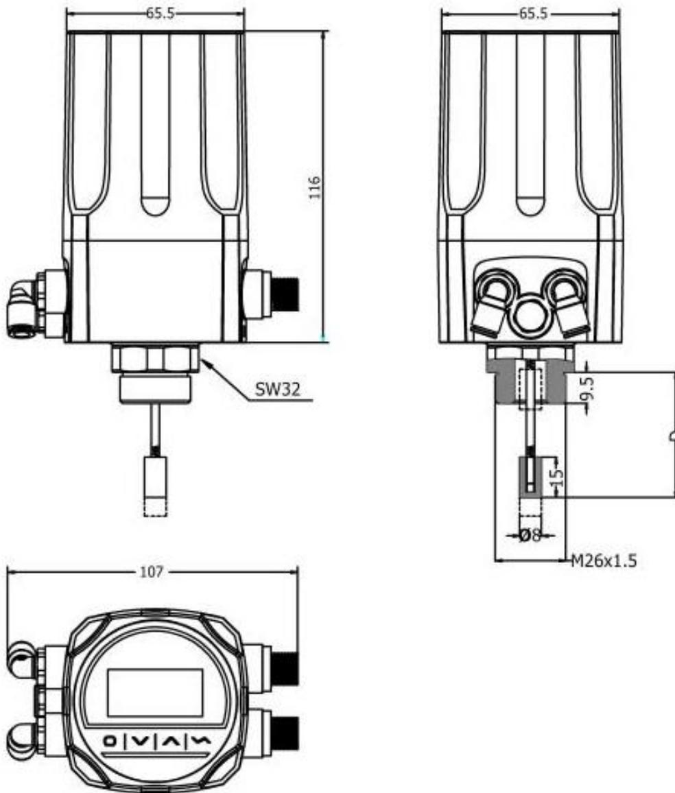
Figure 3. Mechanical dimensions
