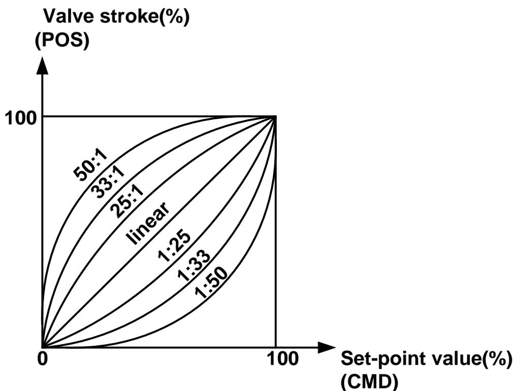
Figure 14. Graph characteristics of linear and equal percentage
