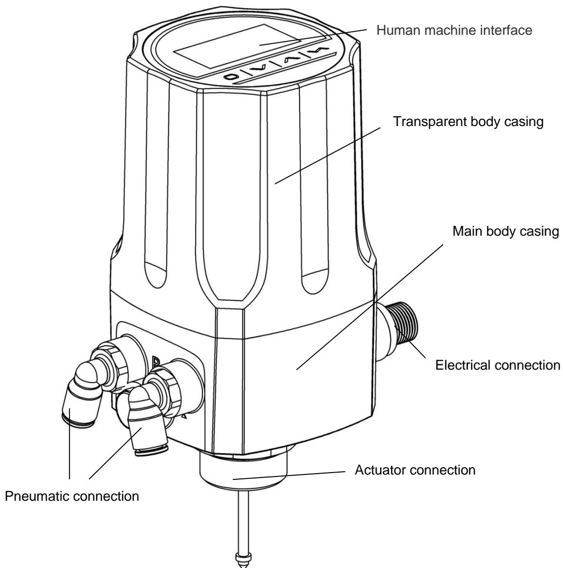
Figure 1. Positioner structure
