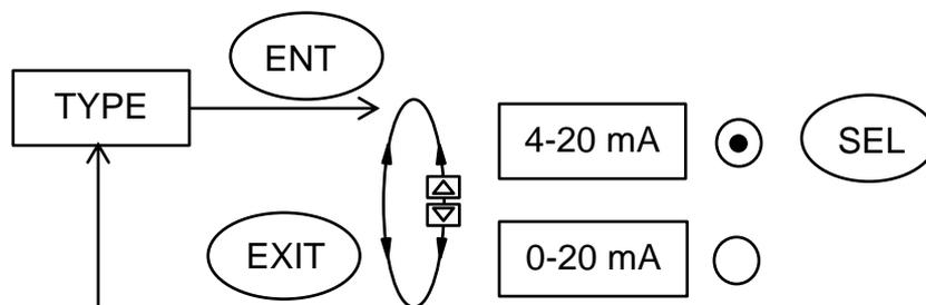
**Figure 27. Operating structure OUTPUT TYPE**
