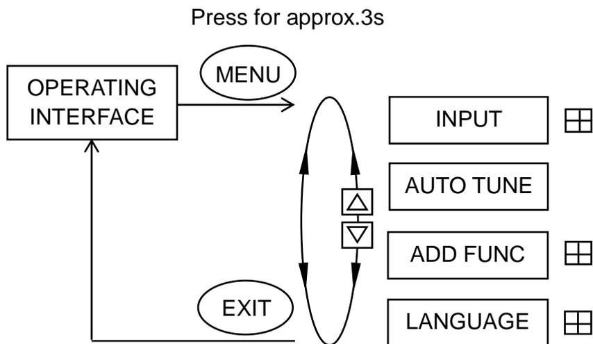
Figure 10. Operating structure main menu
