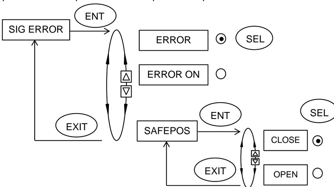
Figure 28. Operating structure SIG ERROR
