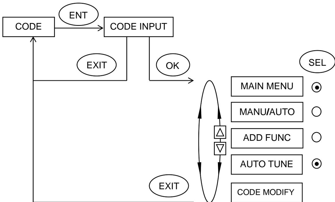
Figure 31. Operating structure CODE
